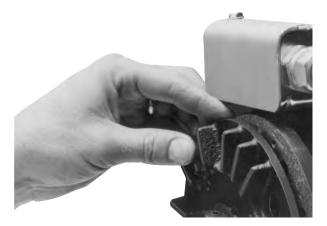
7. Attach the new friction material segments to the brake with the screws through the appropriate access holes. Apply one drop of Loctite (grade 290 or equivalent) to each screw.
