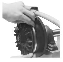
Attach the new armature segments to the cast iron carrier with hex cap screws, lockwashers and washers. Apply one drop of Loctite (grade 290 or equivalent) to each screw. Tighten to the appropriate torque for your size unit.
