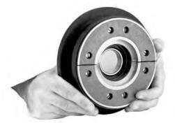
4. Tighten the mounting screws to the machine frame to the appropriate torque for your size brake.
